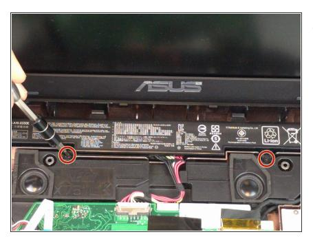
Remove the two 6.6mm Phillips #00 screws holding the battery in place.
