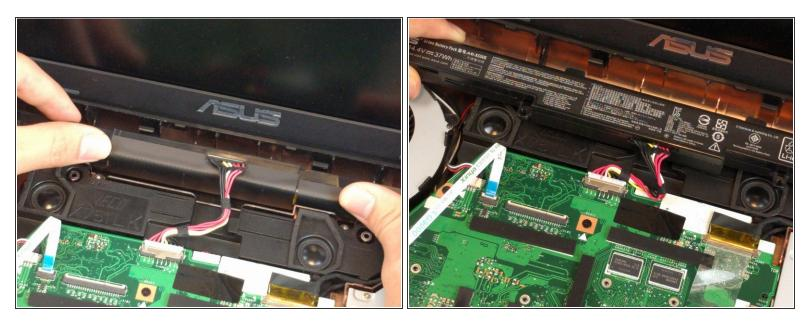
• Lift the battery from the cable-side to maneuver it around the plastic clips.
