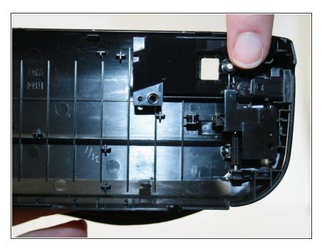
Lift up on the little tab indicated in the picture and push away from the camera in order to remove the record button.
