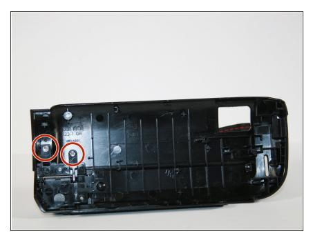
Unscrew the indicated screws and remove the piece it was holding in place.
