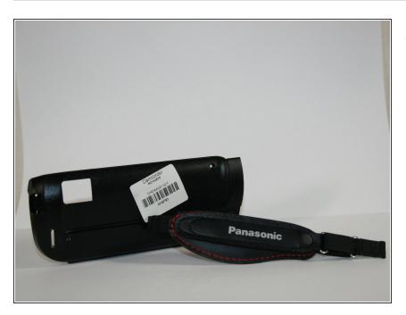
Pull the handle straps out of their holes to remove the strap.
