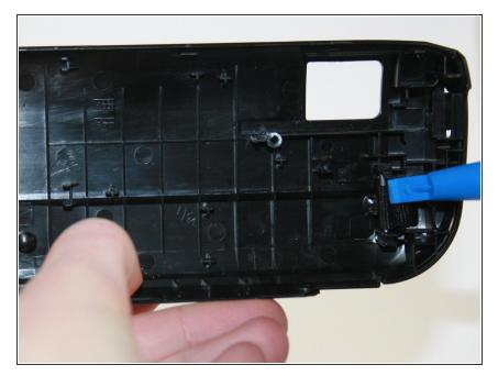
Use the plastic opening tool to pry the little metal bar out of place in order to release one side of the hand strap.
