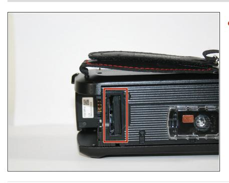
Open the port and push on the SD card to remove it.
