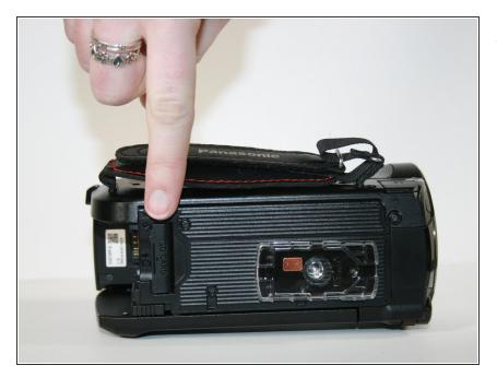
Locate the SD card port on the bottom of the camcorder.
