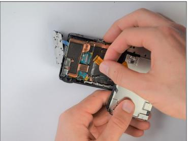
• Carefully unplug ribbon connector to fully detach LCD screen assembly from camera
