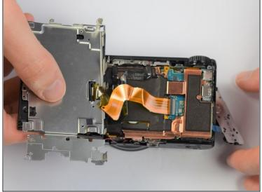
• Remove back panel assembly while still keeping ribbon cable attached
