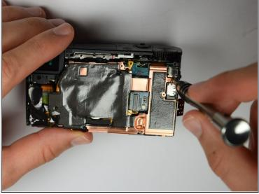
• Remove remaining screw which holds the copper casing in the camera
