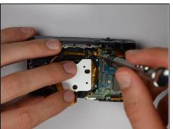
Using Philips Screwdriver, remove the four screws as marked on the picture
