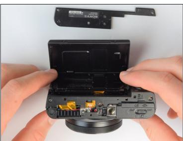
• Using the plastic opening tools, carefully pry off the bottom plate.
