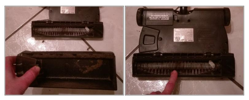
Remove and empty dust tray; make sure to clean any debris built up.
