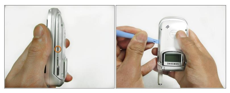
Locate the tabs on either side of the phone. Pull the outer case away from each tab with the plastic opening tool.
