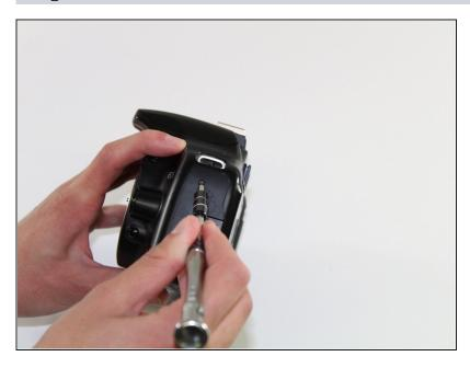
Using the PH000 screwdriver head, remove one 4 mm screw on the left side of the camera (from the LCD screen).
