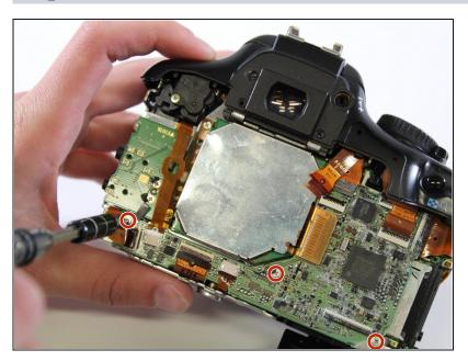
Using the PH00 screwdriver head, unscrew the three 3mm screws.
