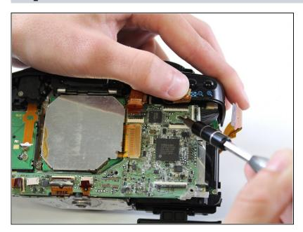
Using the PH00 screwdriver head, unscrew the last 4mm screw from the motherboard.
