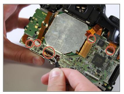
Disconnect the five cables attached to the motherboard by gently pulling with tweezers.
