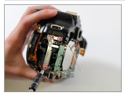
Using the PH00 screwdriver head, unscrew the three 3mm screws on the left side of the camera.
