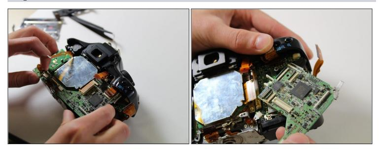
• Remove motherboard by gently lifting out with fingers.
