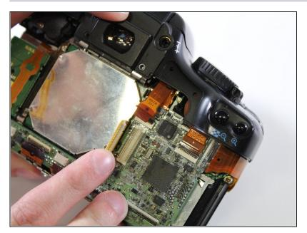
Remove tab from base by lifting up with finger.
