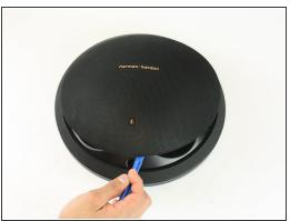
Using a plastic opening tool, pry off the front grill by wedging it in the notch on the front of the device.
