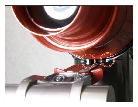
Locate two visible white clips between the main body and the cyclone.
