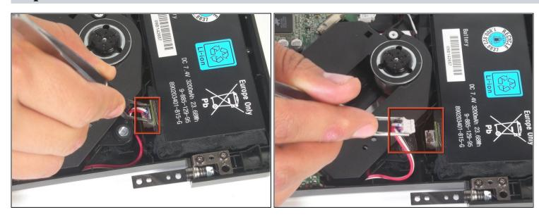
• Remove the white and red wires from the battery by pulling on the base with <u>tweezers</u>.
