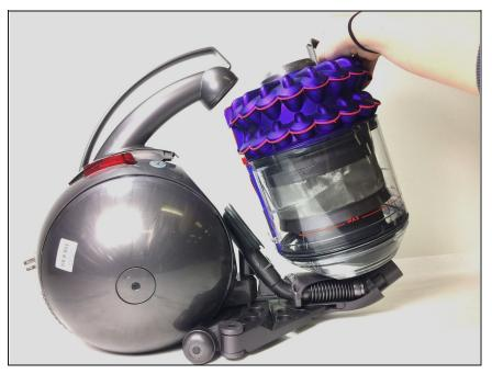
Remove the canister by lifting it out.
