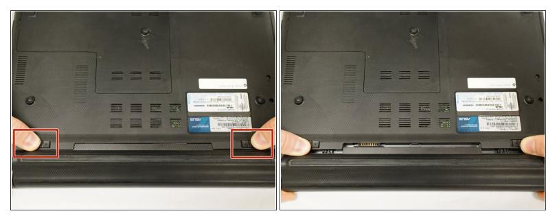
With the laptop battery facing away from you, use your thumbs to push both sliders toward the center of the device. You will hear a soft click. Be careful, the sliders may slide back and pinch your thumbs.
