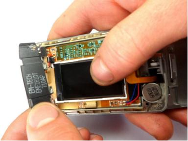
Remove the ear piece from the phone by lifting it using a plastic opening tool.
