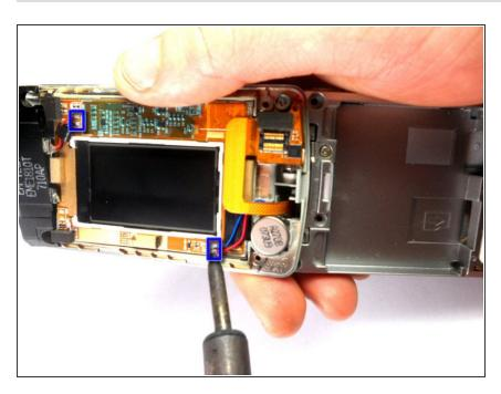
Desolder the wires connected to the LCD board using a soldering iron
