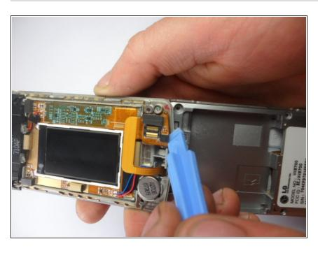
Disconnect the Ribbon connecting the two pieces carefully with the plastic opening tool.
