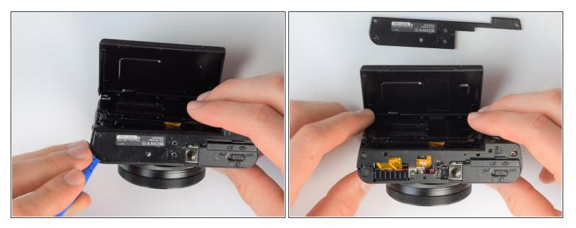
• Using the plastic opening tools, carefully pry off the bottom plate.
