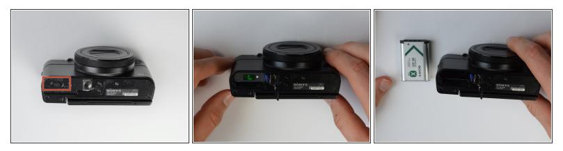
Remove battery by sliding the tab to open the cover
