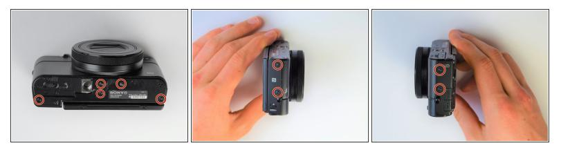
• Using the screwdriver, remove all screws (black 2.5mm) from outermost layer of the assembly.
