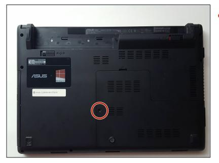
Flip the laptop so that it is upside down and locate a screw near the middle of the laptop. Remove the 8 mm PH0 screw.
