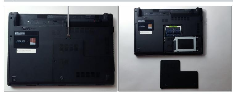
• Use a spudger or opening tool to remove the L shaped section of the back cover.
