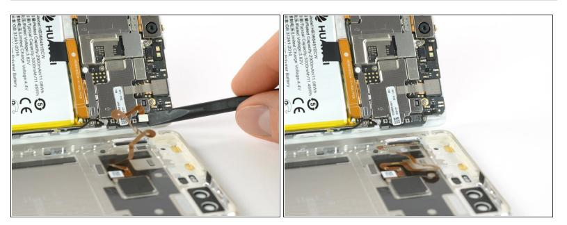
Disconnect the fingerprint sensor using a spudger.
