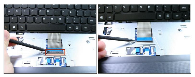
• Push the keyboard connector latch upwards with the spudger.
