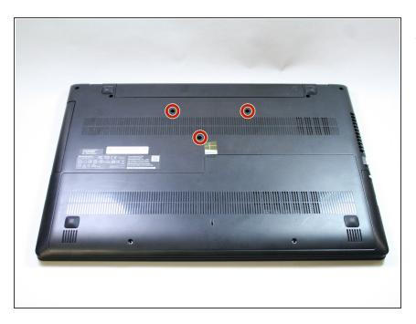
• Unscrew the three 6mm Phillips #1 screws from the upper back cover.
