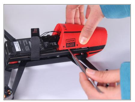
Take the metal spudger, to remove the double stick tape from the foam.
