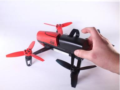
While holding onto the nose, gently pull the battery away from the nose.
