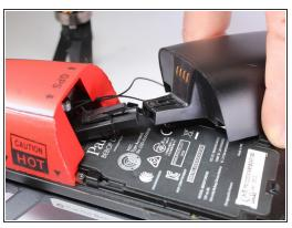
Once the battery is separated from the nose, push down on the connector and pull the battery away from the connector.
