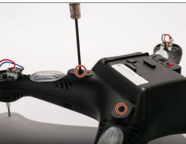
Remove four 9 mm screws located where the legs originally are placed. (Use a thin head screwdriver)
