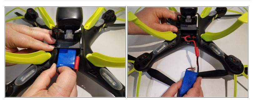
Carefully pull out battery, pulling out wires first.
