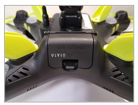
Find door on the underside of drone.Open the door.
