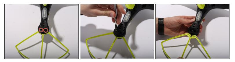
Remove Blade Guards by unscrewing two 13 millimeter screws using Philips #0. Pull out the guards. Repeat the steps for the other three corners.
