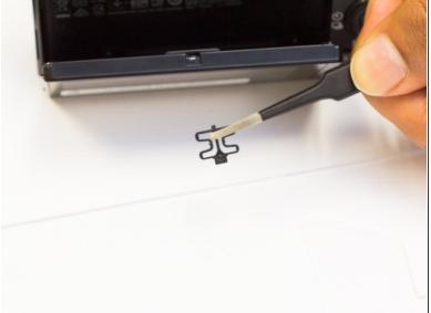
Carefully remove the clip located at the top of the screen.
