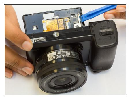
Flip the camera so that it is bottom side up. Pry off the inner support plate.
