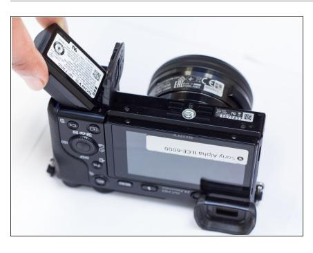
Once the battery is free, you are able to take the battery out of the compartment.
