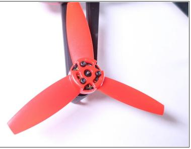
While holding the propeller in place, rotate the tool counterclockwise until the screws are aligned with the holes on the propeller.
