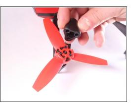
Using the propeller removal tool (included with the Parrot Bebop Drone), line up the holes with the protruding screws.
