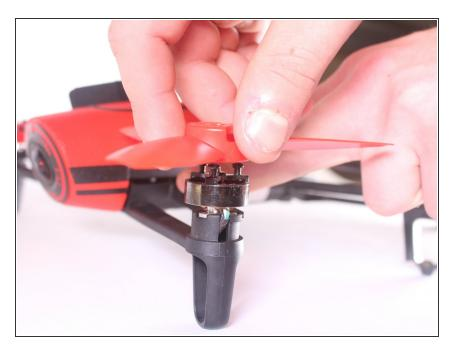
While gently pushing down on the arm of which the propeller is attached, pull the propeller up off the motor.
