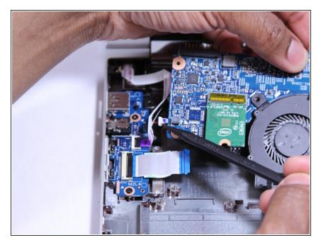
Using a Heavy Duty Spudger, disconnect the black and red RTC battery cable on the left side of the system board (motherboard).
