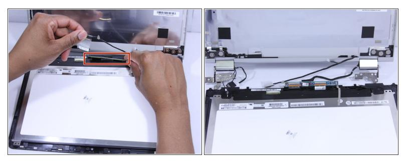
Lift the circuit board out of the way to expose the wire underneath. Remove the wire from the base of the laptop.
