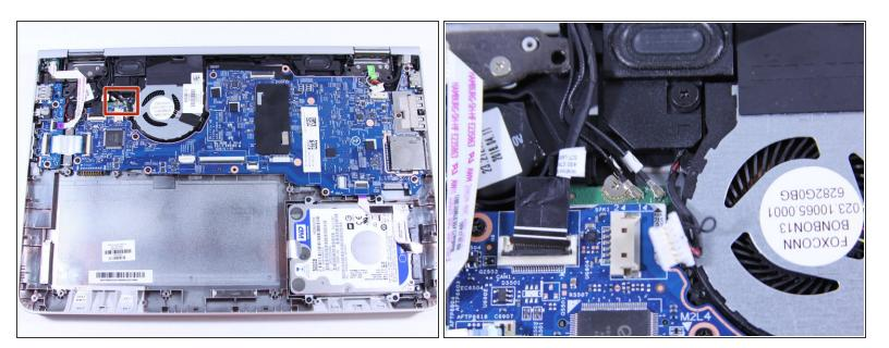
Pull the clipped cables from system board (motherboard).
