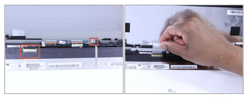
Peel off the adhesive tape and remove the connected cable from the screen.
