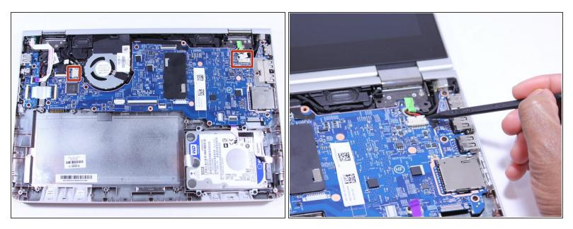
Disconnect the fastened cables from the system board (motherboard) by carefully pushing the cable's plastic edges using the Heavy Duty Spudger.
