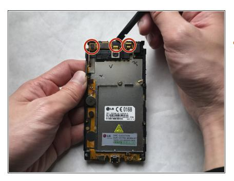
Lift the three connectors using the plastic spudger.
