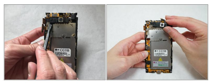
• Starting from the right, remove the attached black mount using the plastic spudger.
