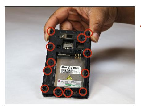
Remove the twelve screws using the Phillips 000 screwdriver.
