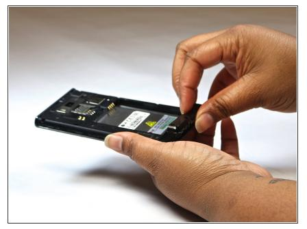
• Remove bottom plate where the charger port is located.
