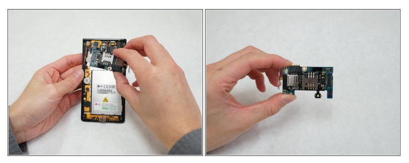
• Detach the mount including both the SIM card and the motherboard from the device.
