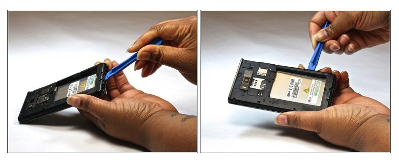
Insert a plastic opening tool between the seams of the device and apply some pressure to lift off the cover.
