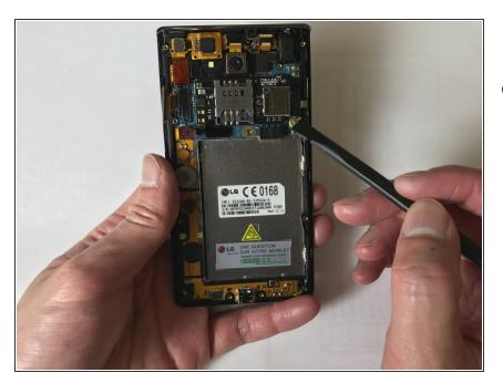
Using a plastic spudger, lift off the wire connector at the right bottom of the board.
