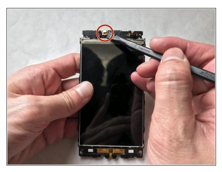
Lift off the connector using the plastic spudger.
