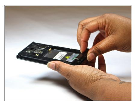
Remove bottom plate where the charger port is located.
