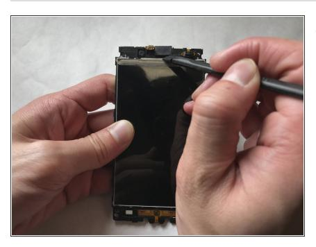
Lift the speaker connector using the plastic spudger.
