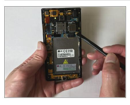
Using a plastic spudger, lift off the wire connector at the right bottom of the board.
