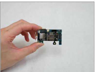
Detach the mount including both the SIM card and the motherboard from the device.
