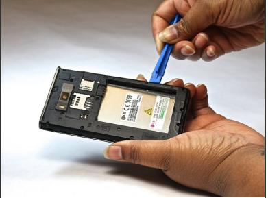
Insert a plastic opening tool between the seams of the device and apply some pressure to lift off the cover.
