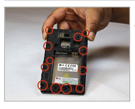
Remove twelve 3mm screws (with the phillips head 000) around frame and near sim and sd cards.
