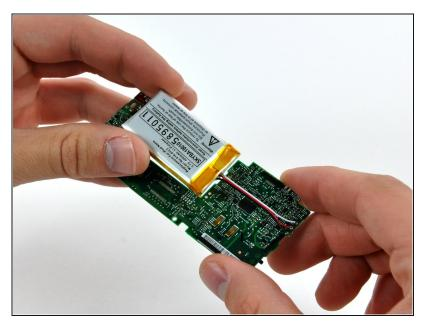
Rotate the battery toward the logic board and place it flat in its void, bending the cables as necessary.
