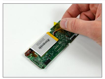
• Peel the orange kapton tape covering the battery leads.
