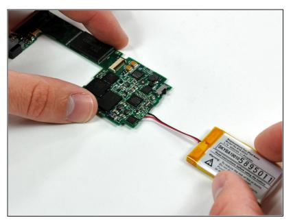
Flip the logic board and battery over so the bare ends of the battery leads are facing up.
