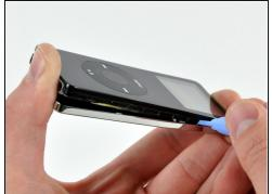
Repeat the same procedure listed in the previous step to free the five clips along the headphone jack side of the iPod.
