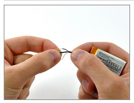
• If present, remove the small piece of shrink tube protecting the new battery's positive lead.
