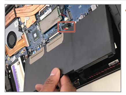
• Unplug the connector highlighted in this picture by pulling it up and out of it's seating, then pull the battery away from the motherboard and remove the battery.
