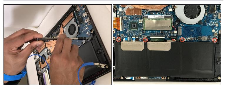
Attach the clip of your <u>anti-static wrist strap</u> to the case of the laptop. This prevents any accidents that could fry the motherboard.
