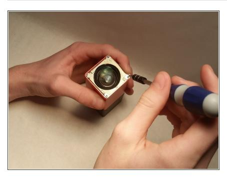
Unscrew the four screws(7.1cm) seen after taking the top off.
