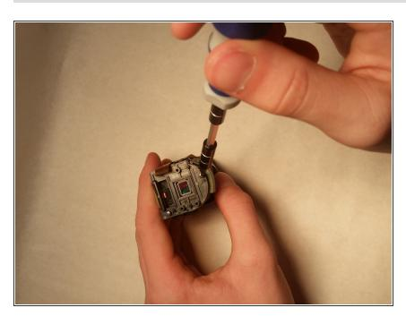
Now you can unscrew the three screws(.5) seen releasing the camera lense from the camera.
