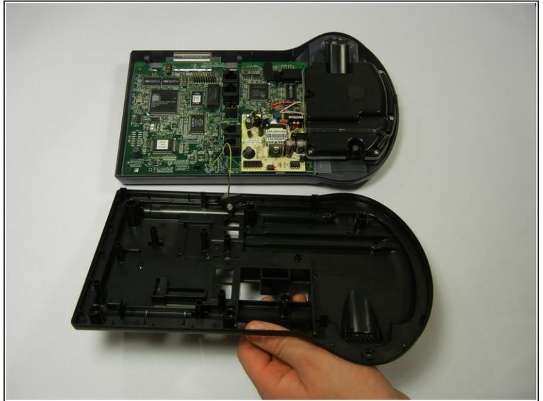
**⚠** Lift up the back cover slowly because there are still wires attached to the circuit board.
