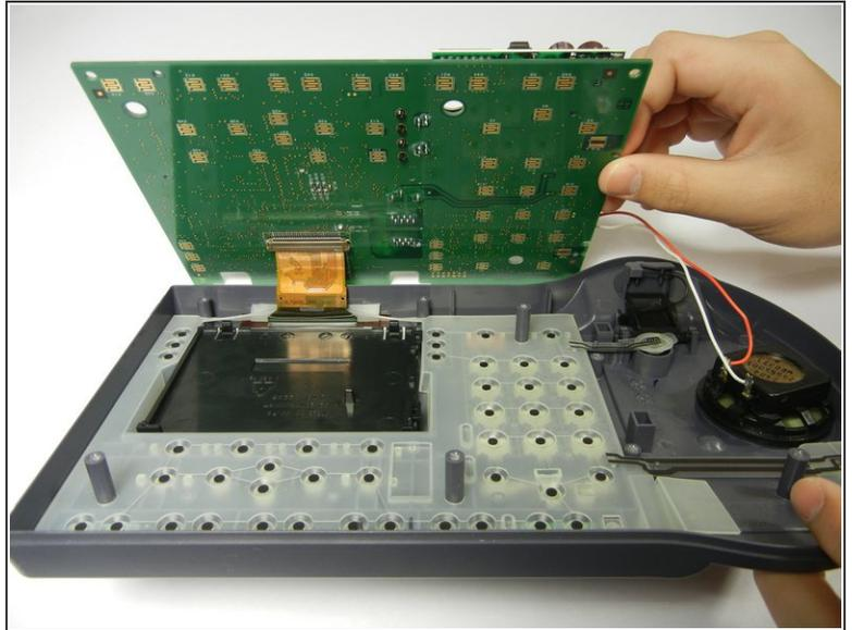
**⚠** There's a brown ribbon still attached to the circuit board and phone case, so don't pull the circuit board completely off just yet.
