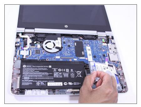
Using the tab provided, lift and remove the hard drive out of the laptop base.
