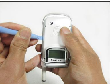
Locate the tabs on either side of the phone. Pull the outer case away from each tab with the plastic opening tool.
