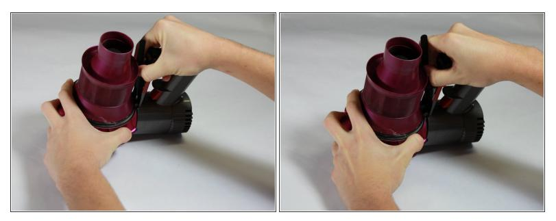
Insert each arm of the tweezer into each white component area and squeeze simultaneously to release the motor from the attached component.
