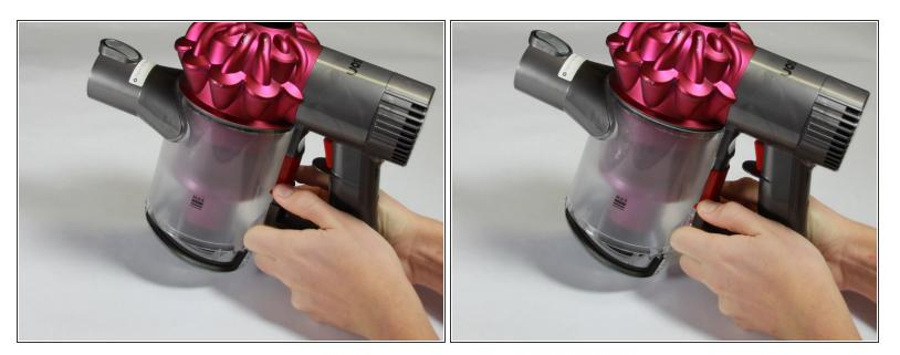
Pull down on the release tab a second time, this time the collection bin should release from the upper vacuum head.
