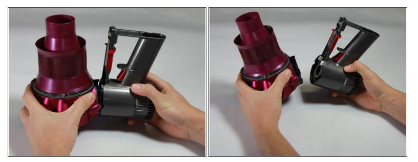
• Detach the motor from the remaining motor head assembly.
