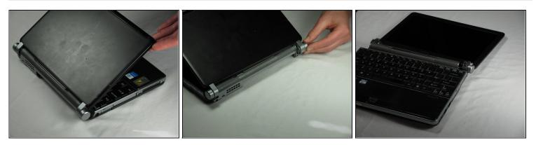
A Mind the wire connections on the bottom right side of the monitor. They are still connected between the monitor and computer.
