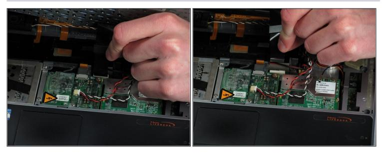
⚠ Disconnect the keyboard by gently pulling on the hard plastic square straight up from the white connector.
