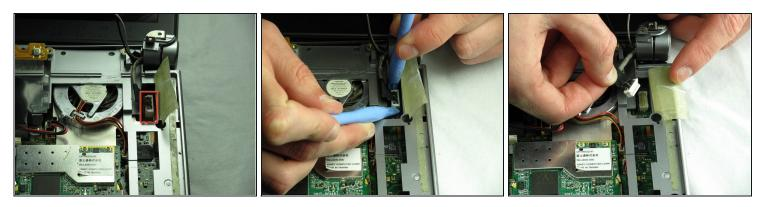
• Unplug the white chip connected to the thicker wire with two smaller spudgers (like a PX3688) by wiggling it back and forth until it pops out.
