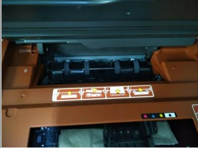
Next, apply pressure on the "clean out door." The door will loosen and allow removal.
