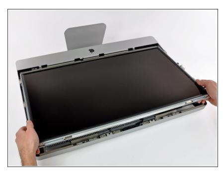
Carefully pull the display toward the top edge of your iMac and lift it out of the iMac case.
