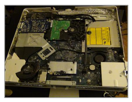
Step one is disassembly, i am not going to go into that in this guide. It is very easily available elsewhere on the internet. That being said, dissassemble to the point where the screen is removed. be sure to remove the lvds cable as well
