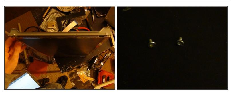
Next we will remove the metal screen brackets. Each side is held on by 2 Torx screws. Remove these screws, remove the brackets, and put them aside. You will need 2 of them later.
