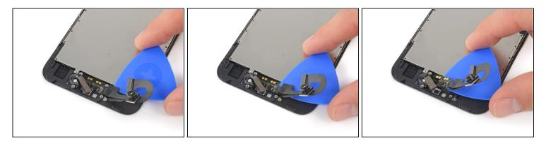
• Use the pick to lift the camera cable up off of the two plastic posts on the front panel and separate it from the last of the adhesive.
