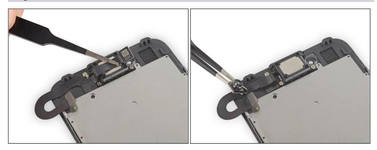
• Lift the front facing camera out of the way to access the earpiece speaker.
