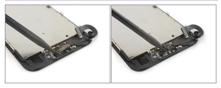
Use a spudger to gently pry the ambient light sensor out of its recess on the front panel.
