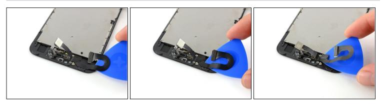
• Slide the pick towards the front facing camera housing, separating the adhesive holding the cable to the front panel. Stop just before the screw posts.
