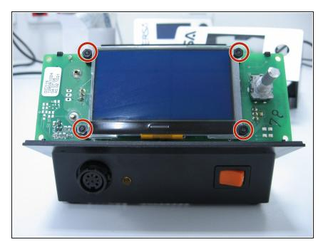
Use pliers or a wrench to unscrew the four plastic nuts holding the display in place.
