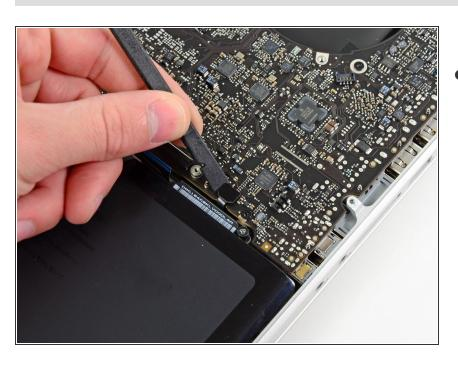
Use the flat end of a spudger to lift the battery indicator connector up and out of its socket on the logic board.
