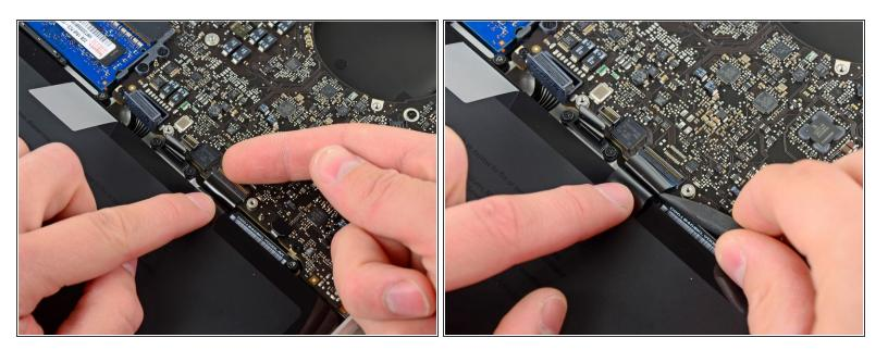
Use your fingernail to flip up the retaining flap on the keyboard ribbon cable ZIF socket.
