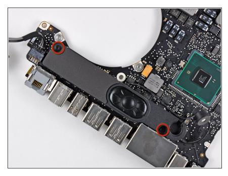
Remove the two 5 mm Phillips screws securing the left speaker to the logic board.
