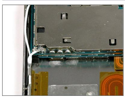
i The solder bead should look like a small dome or hemisphere. If it is flat or jagged, simply place the soldering iron back on the solder to re-melt it and then pull the soldering iron away. It may require a little more solder if this does not work.
