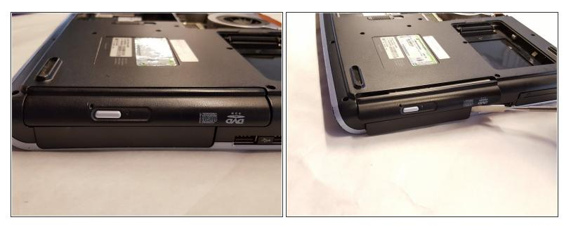
Use the plastic spudger and insert it into the side of the CD drive and push outwards to pop the drive out of place.
