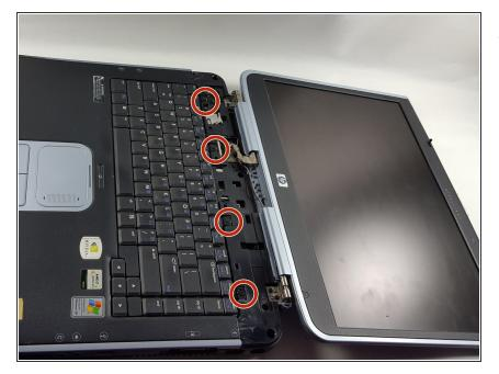
Use the Phillips #0 screwdriver again, unscrew all four Phillips PM 2.5X13.0mm screws from the top of the keyboard and set aside.
