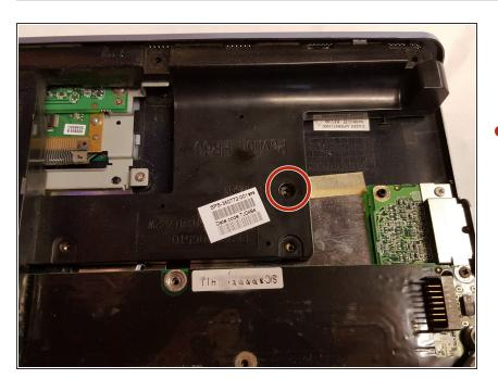
Unscrew the one Phillip 2.5X6.0mm screw using the #0 Phillips again holding the speaker into place but do not remove speaker
