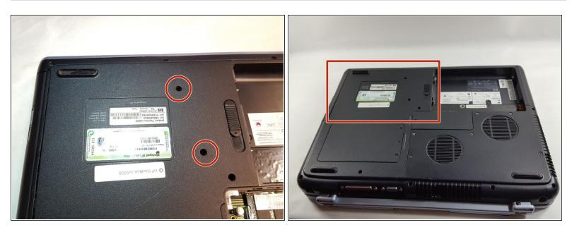
Unscrew the two Phillip PM 2.5X6.0mm screws in the top right that hold the optical cover in place using a Philips #0 screwdriver.
