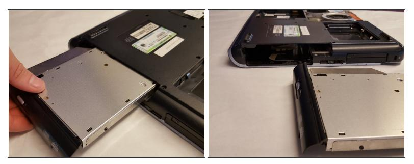
• Using your hands, firmly grasp the CD drive and pull outwards until it is completely removed.
