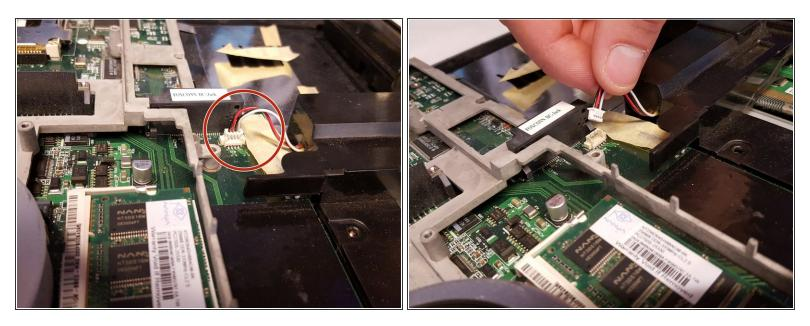
• Using your fingers, firmly grasp the wires that connect the speaker to the board and gently pull the cable away from the connector in the same direction that the wires are running.
