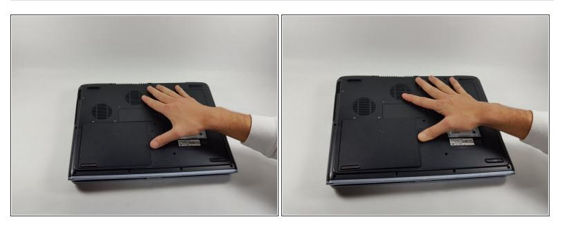
• Press and slide up the battery release tab with your thumb until the battery pops out of place.
