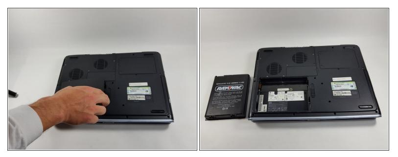
• Using two fingers, pry the rest of the battery out of the socket.
