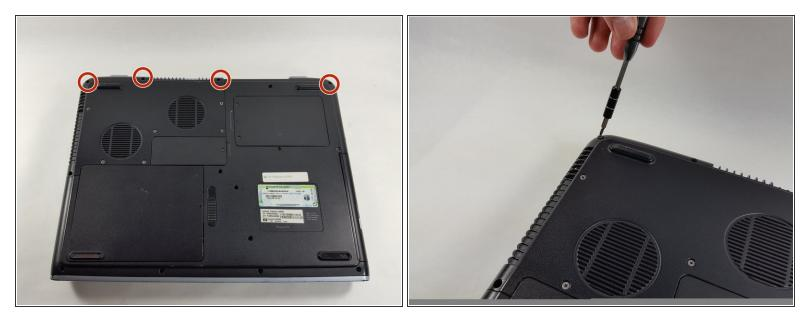
Using a Phillips #0 screwdriver, unscrew all four Phillips PM 2.5X13.0mm screws and place in a secure area until the end of the project.
