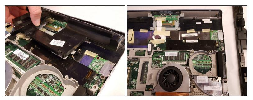
Grasp speaker assembly firmly and pull towards you and up to remove the speaker completely from the laptop.
