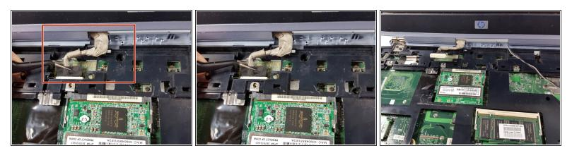
Using the tweezers, gently squeeze and pull backwards on the display cable until it is disconnected.
