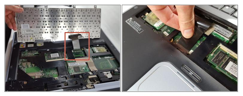
• Gently slide out the connecting cable from the laptop to the keyboard.
