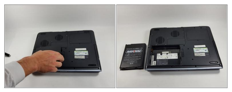
• Using two fingers, pry the rest of the battery out of the socket.
