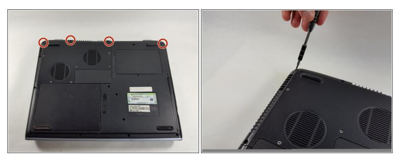
Using a Phillips #0 screwdriver, unscrew all four Phillips PM 2.5X13.0mm screws and place in a secure area until the end of the project.
