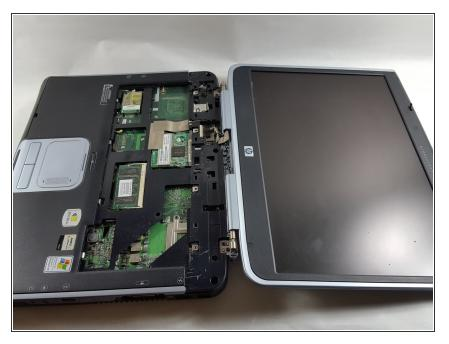
• Completely remove the keyboard from the rest of the laptop.
