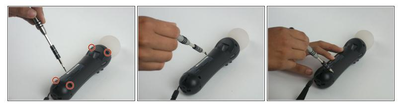
• Using a Phillips #0 screwdriver, remove the four 10mm screws located on the back of the device.
