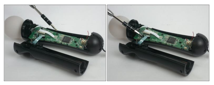
• Remove the two 1.2mm Phillips #1 screws.
