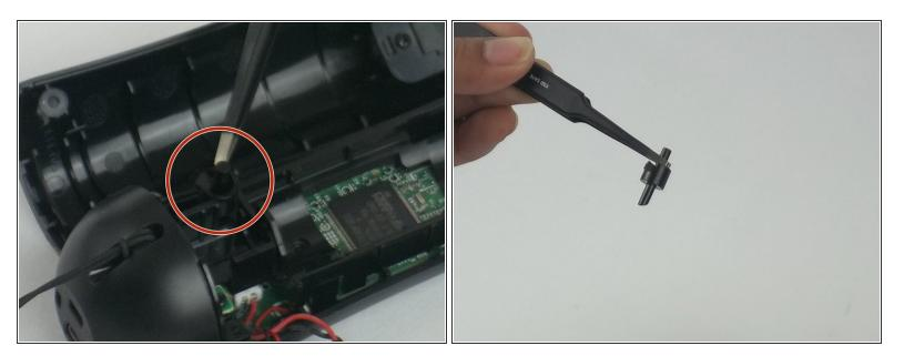
Using tweezers, remove the small piece with a cylindrical top that is located to the left of the inner plastic frame.
