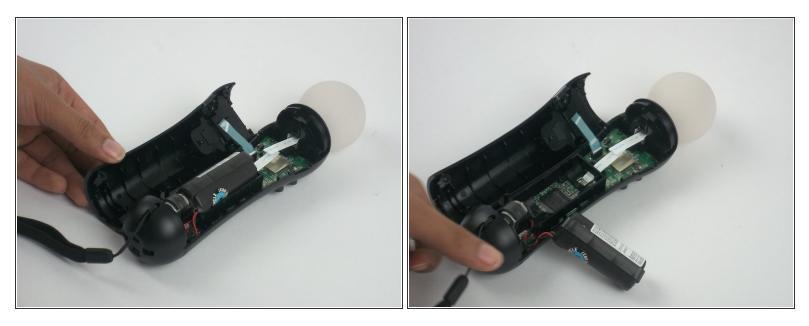
• Once the device is opened, lift the battery out of the black plastic holder.
