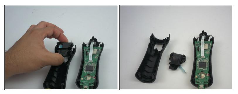
• Remove the trigger button from the controller.
