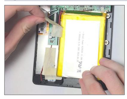
• Remove masking tape from the battery.
