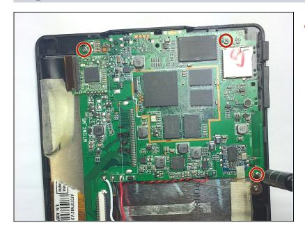
• Use the nut driver and J00 bit to remove the three 4 mm screws.
