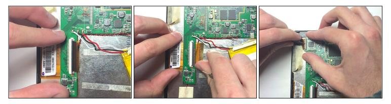
• Remove the two ZIF connectors attached to the motherboard by flipping up the black tabs before pulling the ribbon cable away.
