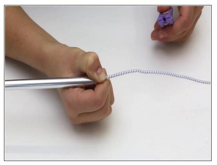
• Hold the shock cord and tension with the help of a clothes pin.
