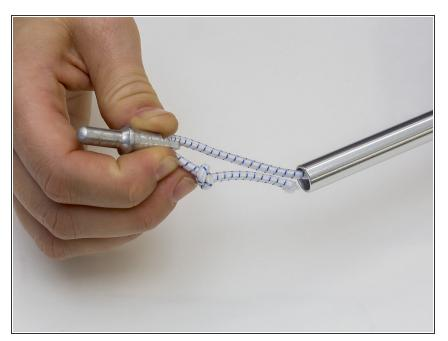
• When the shock cord is hanging out of the tent pole with a fair amount of excess, insert the pin back into the pole at the other end.
