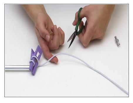
Now attach the end pin to this side of the shock cord, tie a knot in it, and insert it into the pole.
