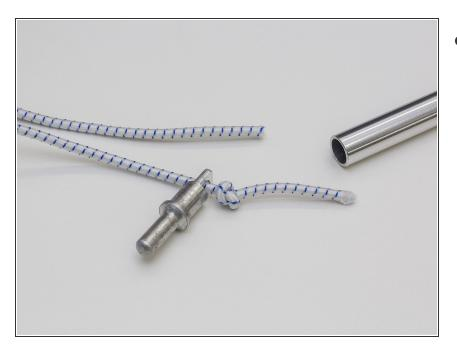
• Attach the new shock cord to the pin and tie a knot in it.
