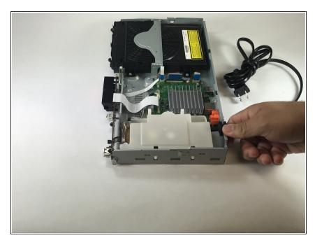
Gently pull on up on the power cord to unlatch it from the metal body of the device.
