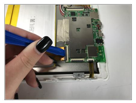
Using the plastic opening tool, lift up the black retaining flap that secures the ZIF (zero insertion force) ribbon connector over the battery to the motherboard.
