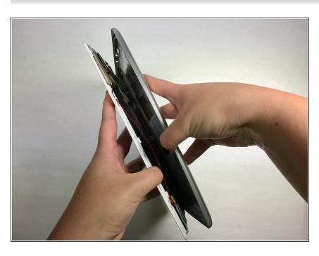
Using an unfolding motion along the top edge of the tablet, carefully separate the front panel from the back case.
