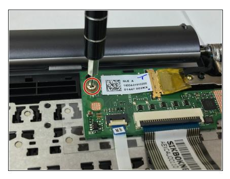
Use the Phillips #00 screwdriver to remove the 4.5 mm screw on the keyboard circuit board.
