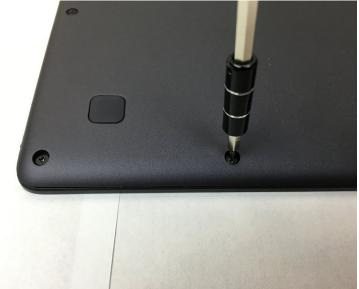
Use a Phillips #00 screwdriver to remove the six 4 mm screws on the underside of the device.
