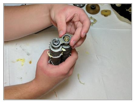
• Remove the metal attachment that holds the two shafts together.
