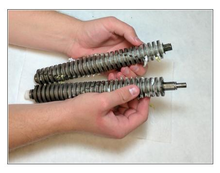
• The shafts can now be pulled apart and any obstructions located between or on each of the shafts can be removed.
